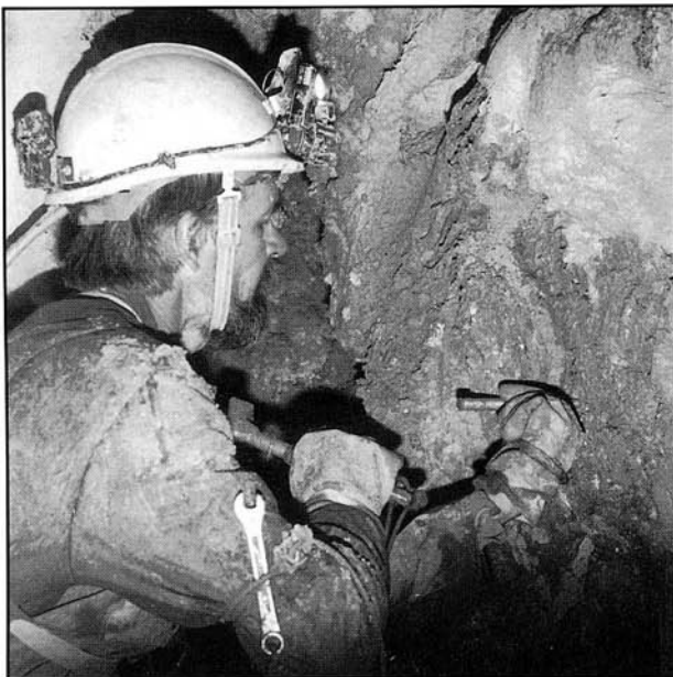
Brian placing spits the 'Bosch-less' way. Dave Dobson
